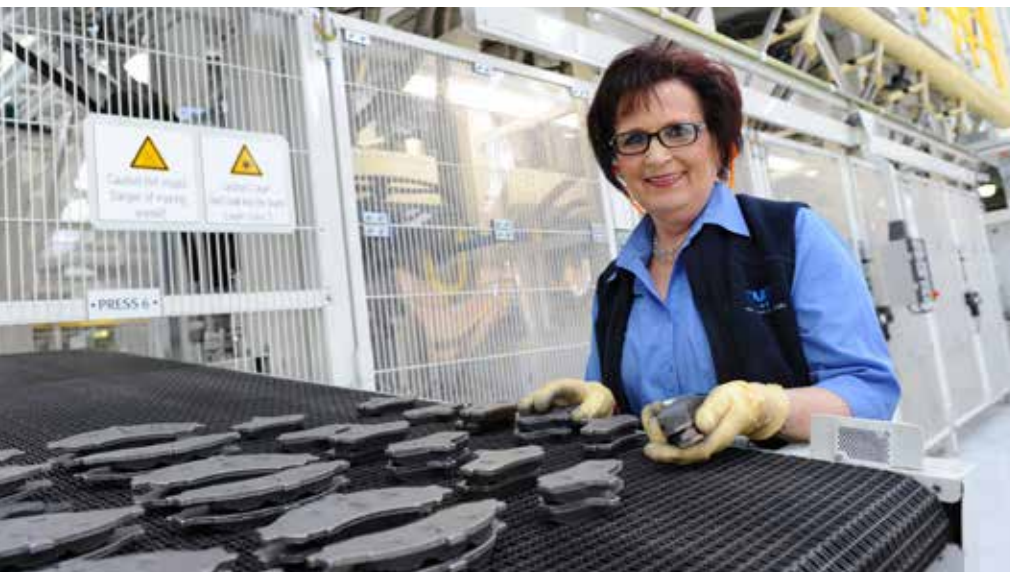
FMP Group Ballarat, manufacturing vehicle brake linings and disc pads.
